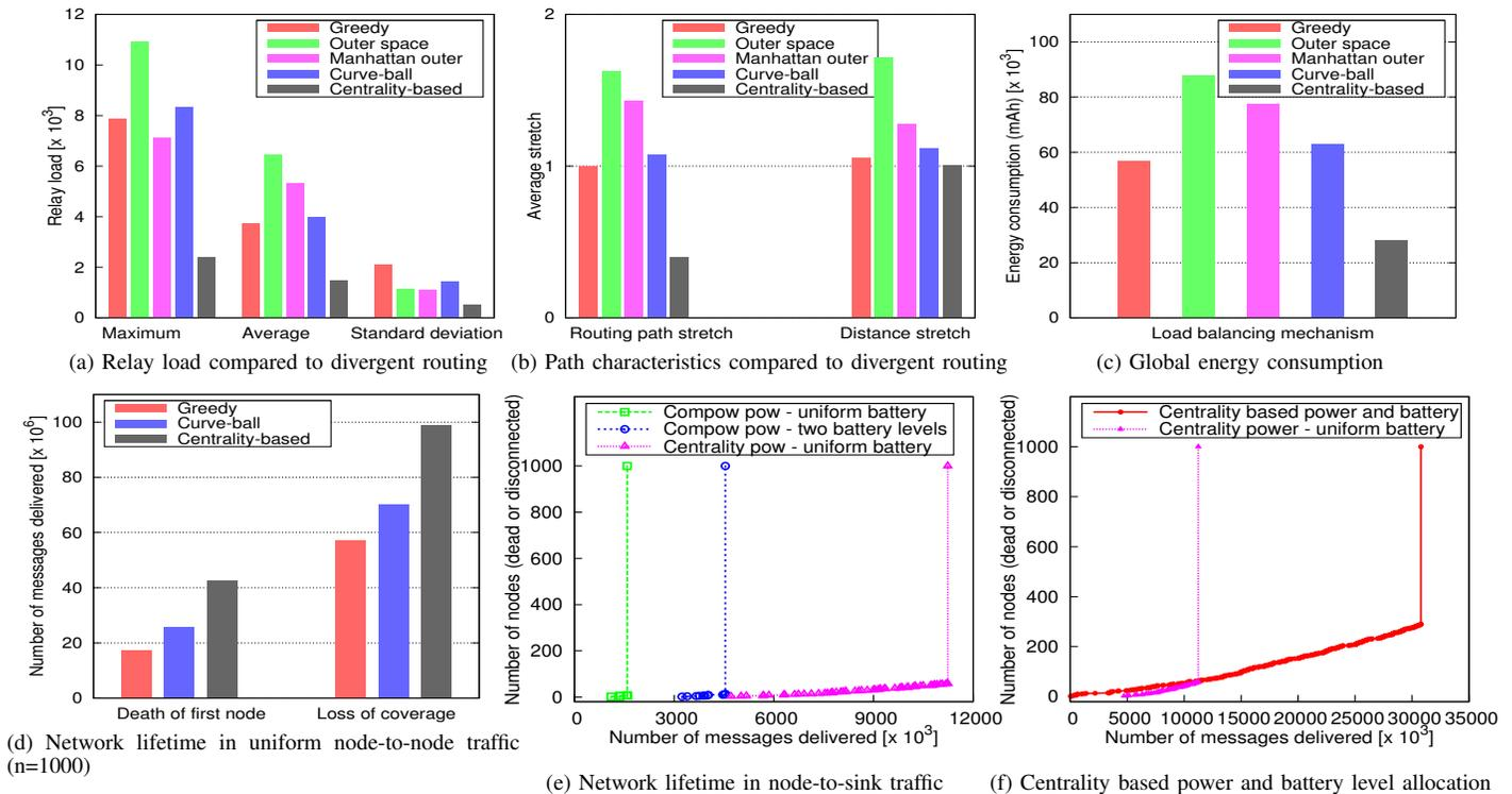
Fig. 3: Effects of centrality based power control on load balancing, energy efficiency and network lifetime
