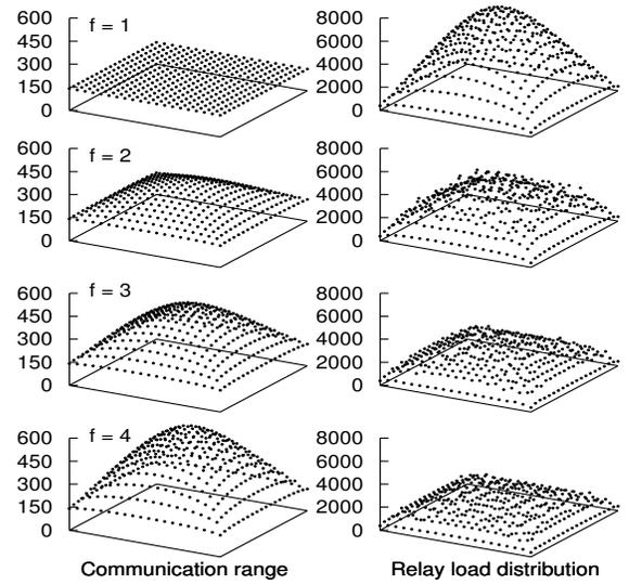
Fig. 2: Effect of growth factor on load balancing in 20x20 grid with uniform traffic
